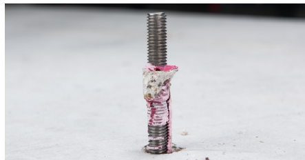
Fig. 3.18: Combined pull-out and concrete cone failure under tension loading
