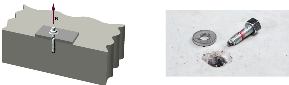
Fig. 3.15: Steel failure under tension loading
