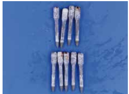
Start of carbon steel corrosion (red rust)
