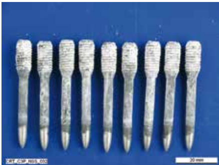
Zinc corrosion (white rust)
