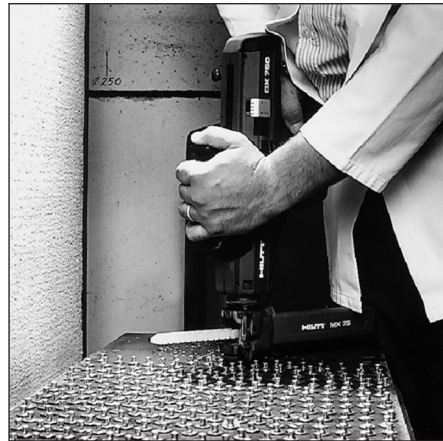
Lifetime testing of the DX powder-actuated tool with nail magazine
