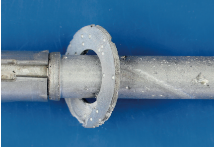
Fig. 5: Example of pitting corrosion on a stainless steel product.
