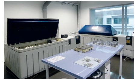
Fig. 13: Picture from our corrosion lab with various corrosion testing chambers.
