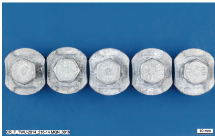
Fig. 18: Connector part with multilayer coating (organic flake topcoat) after ten weeks in the ISO 20340 test with UV radiation.
