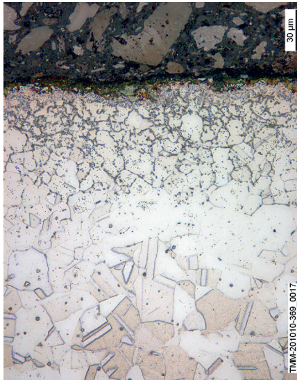
Fig. 11: Scanning electron micrograph image of a selective attack Welded zone of a 1.4401, (A4, 316) material.
