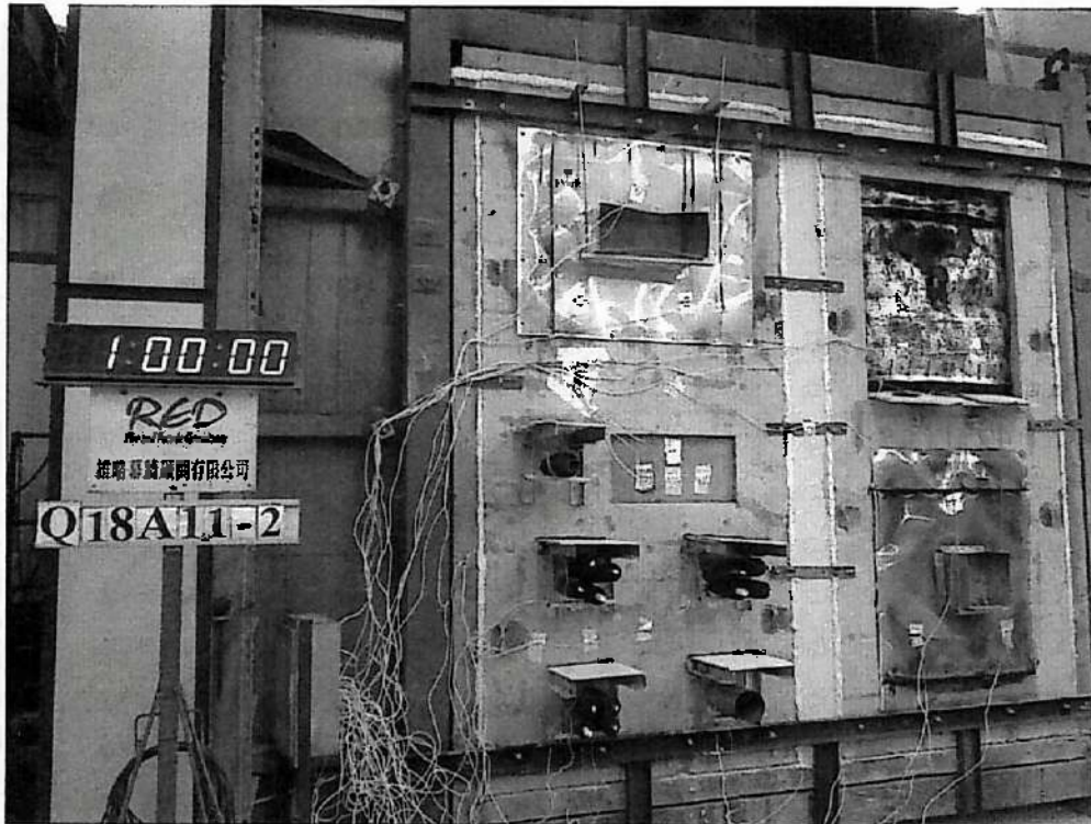
Photo 3: The unexposed face of the specimens after a heating period of 60 minutes.
