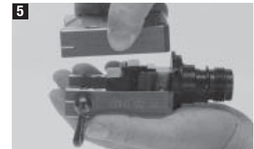
5 Joint the upper and lower housing and secure the 4 locking screws M6x30 using Loctite and an Allen key.
