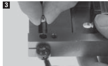
3 Insert the axle with locking lever in the bore as shown taking care not to lose the ball bearing.
